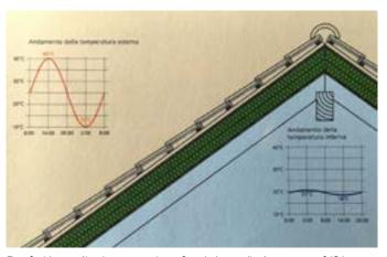
Roof with amplitude attenuation of and phase displacement of 12 hours
