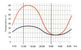
Temperature under the roof cover External temperature
